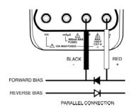
Normal forward voltage drop (forward biased) for a good silicon diode is between 0.4V to 0.9V. A reading higher than that indicates a leaky (defective) diode. A zero reading indicates a shorted (defective) diode. An "**OL**" indicates an open (defective).
